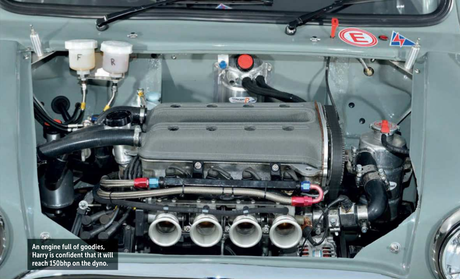
16-valve head fitted with Specialist Components kit.
