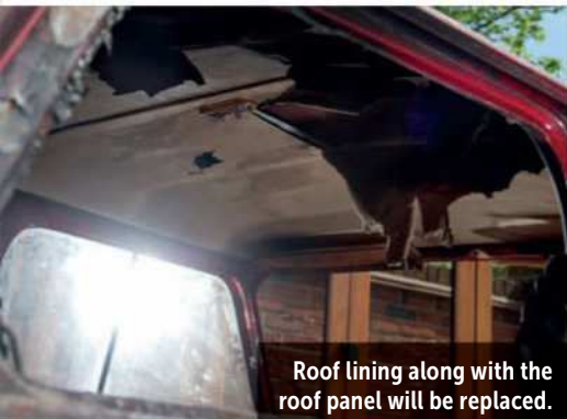
The interior was also caught in the fire.
